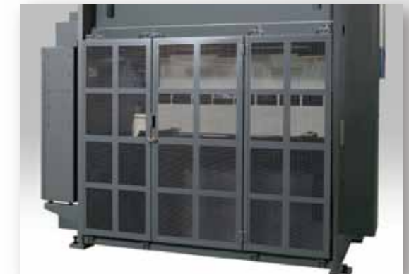
Intrusion to movable parts from the rear part of the machine is guarded to prevent unexpected hazards and ensure safe work. When the rear safety fence is opened, the machine is inoperable until the interlock is released.
