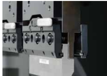
The one touch clamp can be opened and closed with the clamp lever and tools can be easily attached and detached.
